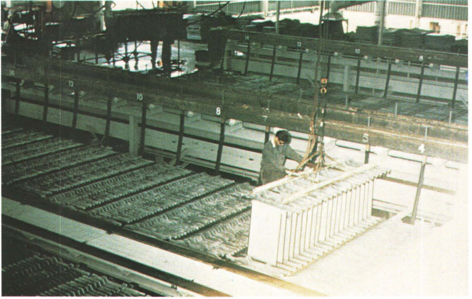
Broken Hill Associated Smelters Pty Ltd Ore smelting and refining at Port Pirie. Interior of Cell Room in Zinc Plant showing cathodes being removed for stripping
