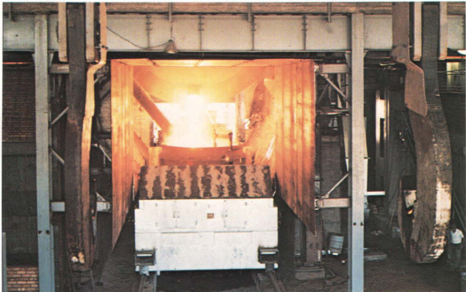
Tapping one of the two furnaces in the Basic Oxygen Steel making (BOS) plant at Whyalla. Each has a capacity of 100 tonnes and a heat cycle of 45 minutes
